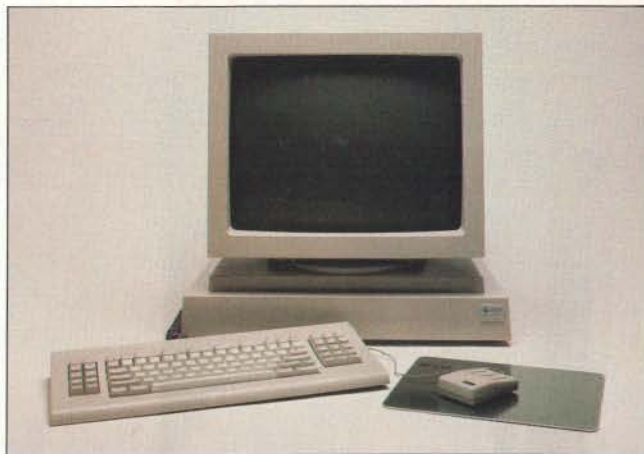
The Sun 3/60 runs at 3 MIPS and can take 24 megabytes of RAM.
